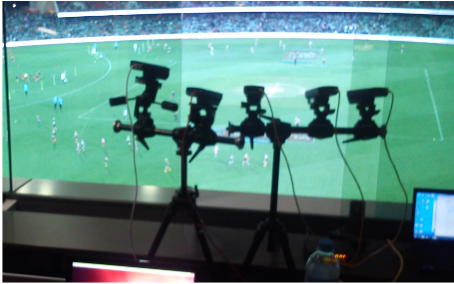
Figure 3.2: The five cameras setup on rig with two tripods overlooking field.
