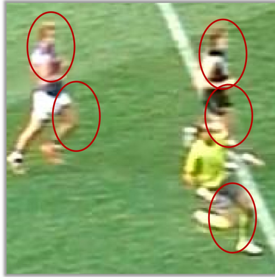
Figure 3.5: Vertical frame problems: Caused by interlacing creating sharp vertical cuts.
