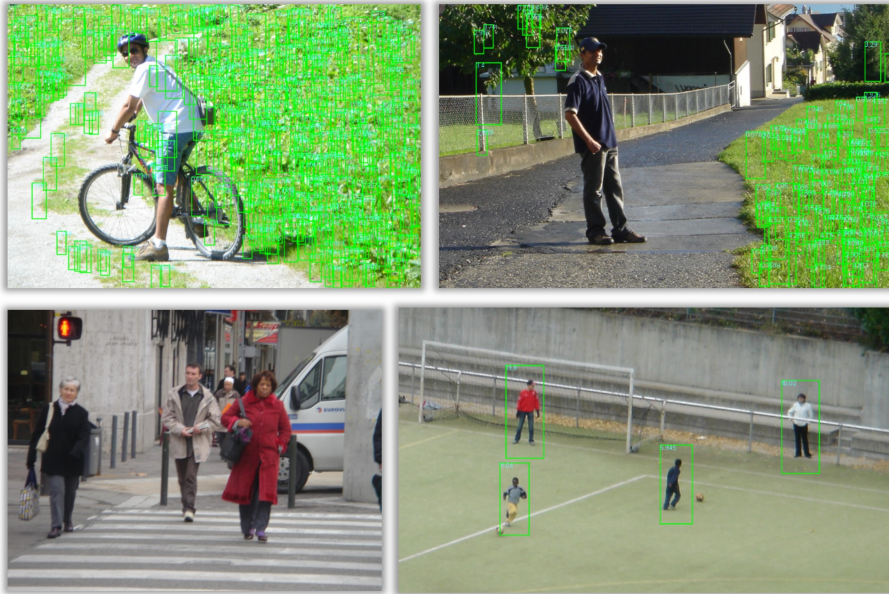
Figure 4.5: The AFL detection results on some selected INRIA test images. Performs terribly on all cases except for the soccer image which is reflective of the AFL problem.
