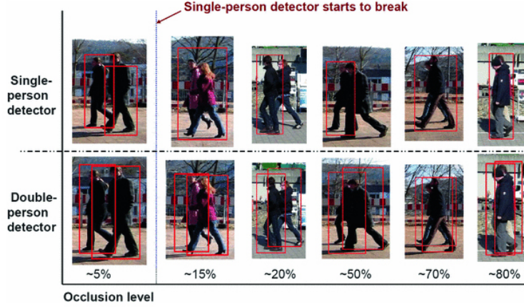
Figure 2.14: Qualitative comparison of single- and double-person detectors for different occlusion levels. Reproduced from [63].
