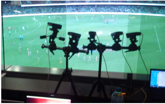
Fig. 3. The five cameras setup on rig with two tripods overlooking field.
